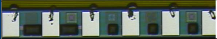
Probe marks misaligned/ out of bond pads
