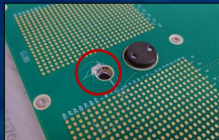
Damaged Probe Card
