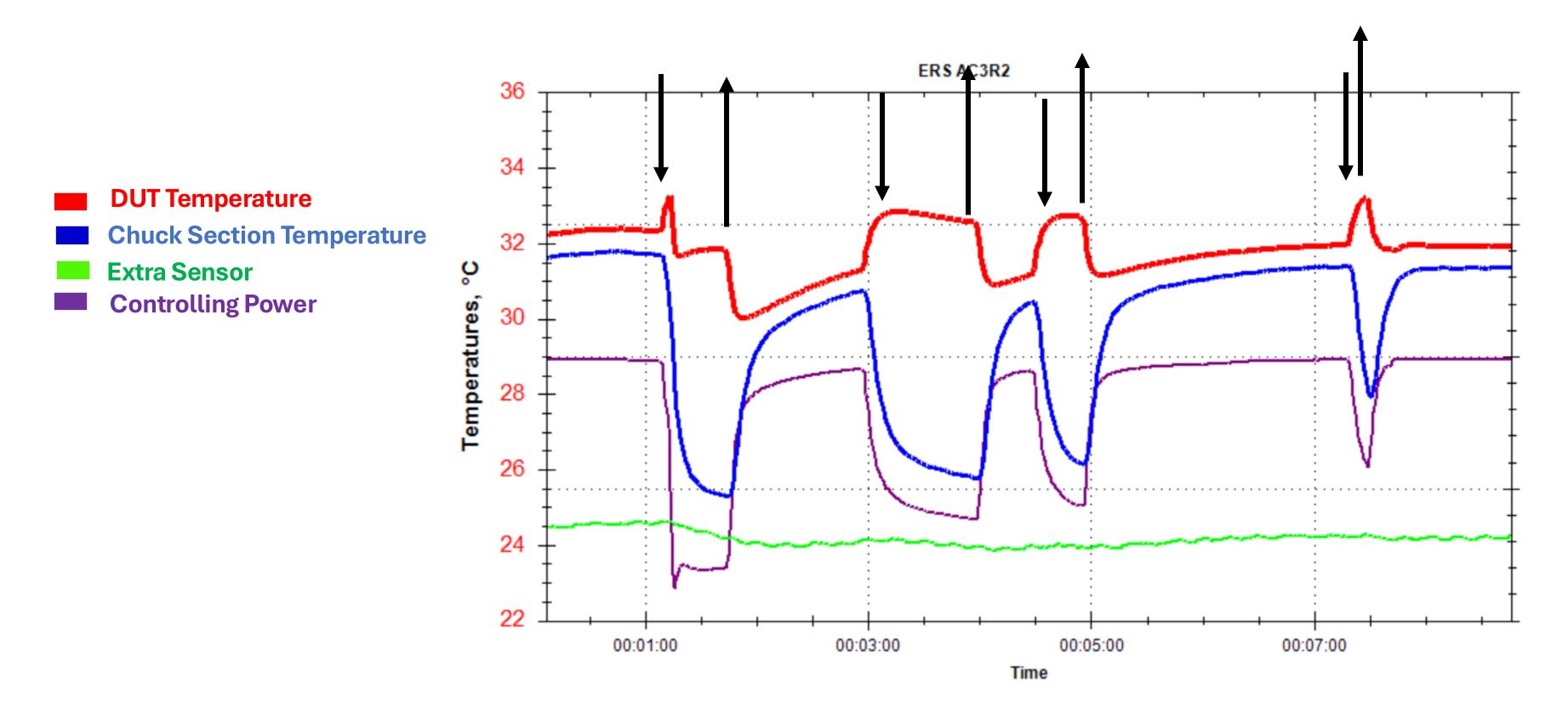
Temperature Difference DUT Power OFF – ON = 33,1-30,5 = <u>2,6°C</u>
