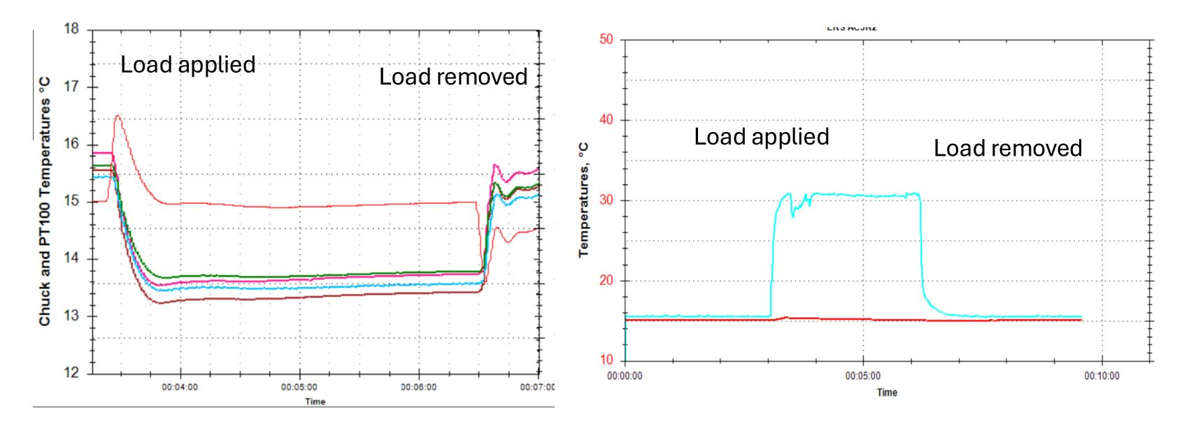
Temperature Difference DUT Power OFF – ON = 32-15 = <u>17°C</u>
