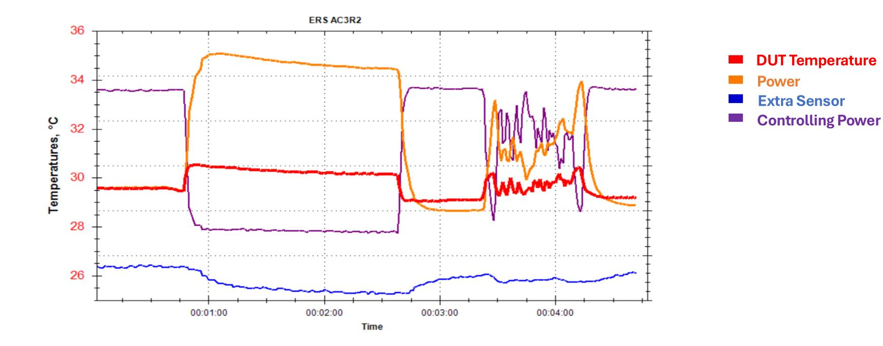
Temperature Difference DUT Power OFF – ON =  $35-30 = 5^{\circ}C$
