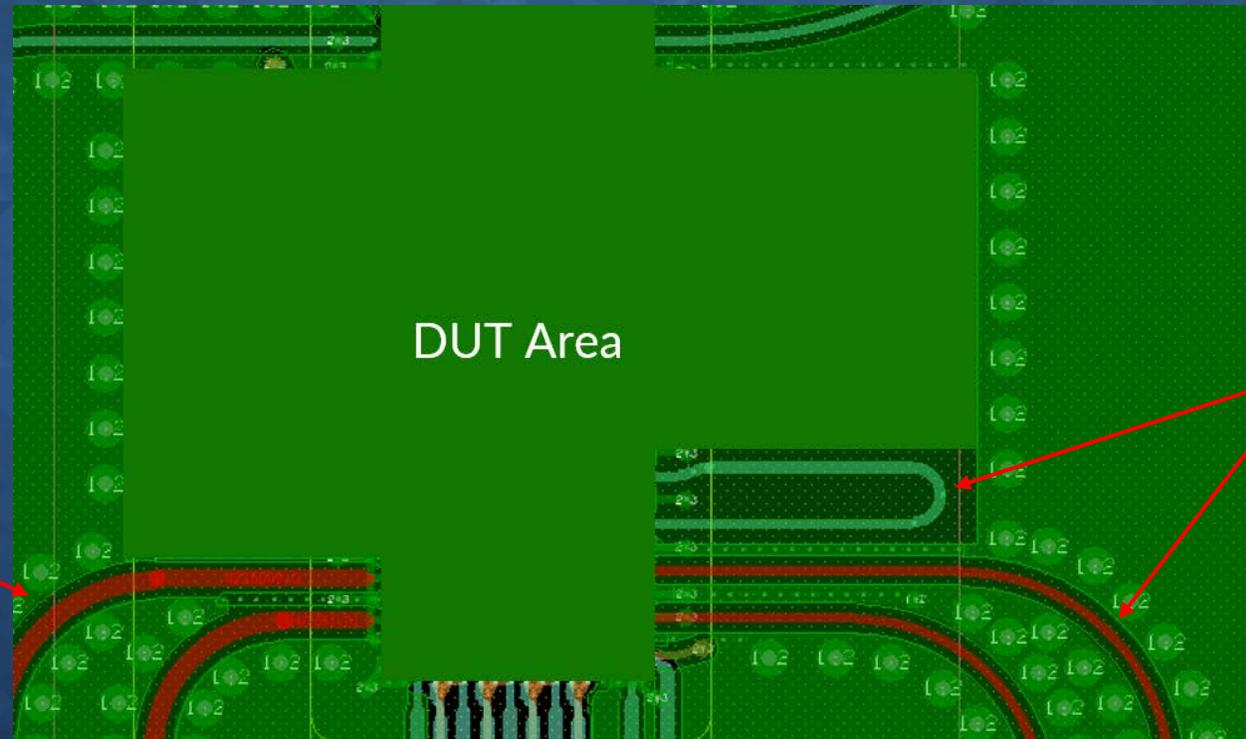
Original trace geometry for 50  $\Omega$  loopback and direct connections
